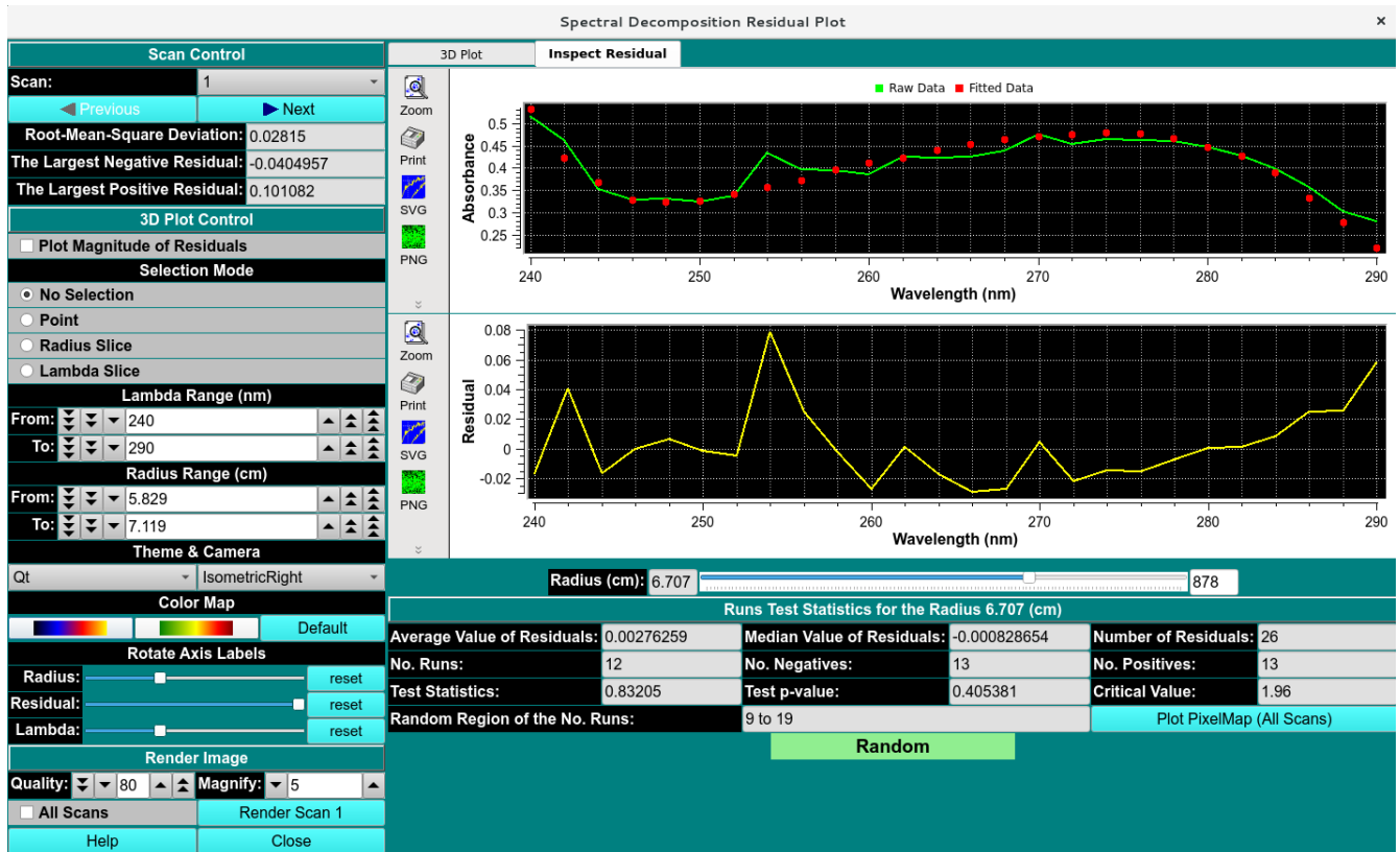
SF 2: Screen shot of the spectral decomposition residual plot in UltraScan demonstrating the fit and residuals at individual radius positions for all wavelengths measured for AAV8.
