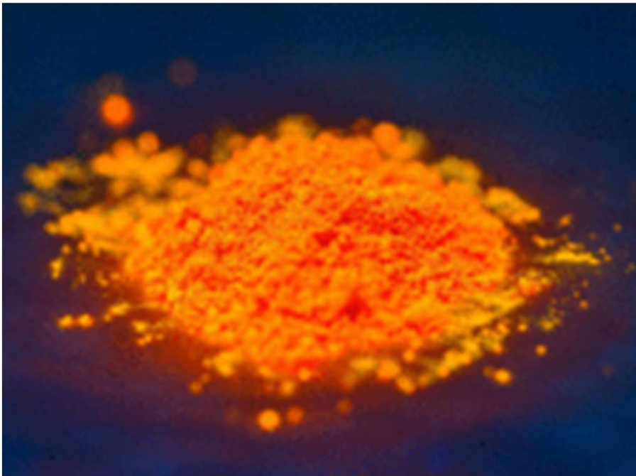
Figure 26. Image of \text{CuInS}_2 quantum dots with an EM radiation emission peak at about 590nm, which appears orange [8].
